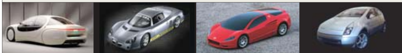
Figure 18: Four carbon-fiber concept cars: From L–R, they are: 1991 GM 4-seat Ultralite (635 kg, C_d 0.192, 0–60 mph in 7.3 s, 84 mpg [2.8 L/100 km] using a nonhybrid gasoline engine); 2002 Opel 2-seat Eco-Speedster diesel hybrid (660 kg, C_d 0.20, max. 155 mph [250 km/h], 94 mpg [2.5 L/100 km], below-Euro-4 emissions); 2004 Toyota Alessandro Volta , 3 seats abreast, by-wire, 408-hp hybrid, 32 mpg, 0–60 mph in <4 s, top speed governed to 155 mph; 2000 Hypercar Revolution show car that mocks up a midsize SUV virtual design (857 kg, 5 seats, by-wire, C_d 0.26, 0–60 mph in 8.2 s, 114 mpg-equivalent with fuel cell).
