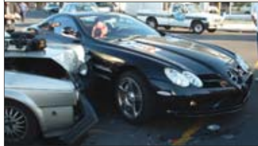
Figure 14: The strength of ultralight carbon-fiber autobodies was illustrated in November 2003 in Capetown, South Africa, when a Mercedes SLR McLaren was rammed by a VW Golf running a red light. The SLR —a 1,768-kg, hand-layup, 626-hp, 207-mph, 16-mpg, street-licensed supercar priced at a half-million dollars—sustained only minor damage despite being hit on the driver's-side door (the photograph shows a carbon side panel popped off). The unfortunate steel Golf , roughly one-fourth lighter than the SLR , had to be towed.
