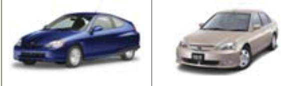
Figure 9: Two mild hybrids competing with the full-hybrid Toyota Prius in the U.S. L: 2-seat Honda Insight , 59–64 mpg. R: The reportedly profitable 5-seat Honda Civic Hybrid , 49 mpg, ~10% share of Civic market. Insight 's successor might resemble the 2003 carbon-fiber concept IMAS —698 kg, C_d 0.20, 94 mpg on the Japanese 10/15 cycle.
