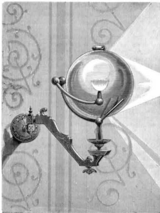
lens and adjustable bracket. The lens is hollow and is filled with filtered water or a solution of salts; its diameter, for general purposes, is about six inches. The bracket consists of an ordinary ground burner and socket, the latter joined to the adjustable or swinging arm. The lens is supported at three points, namely, by the lower or stationary half of the swinging arm and by two small supports projecting from the upper part of the socket.
