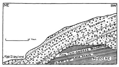
FIGURE 4.—Section of small Promontory on Coast 2 Miles West of Clallum. Showing unconformity between the Miocene and Pliocene.
