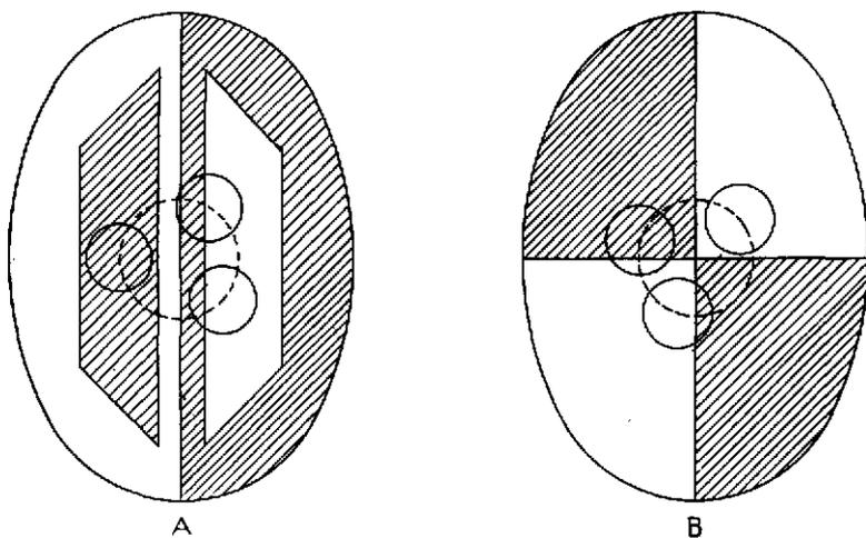
To show how the Lummer-Brodhun field (A) is cut by the attachment; also a four-part field (B).
