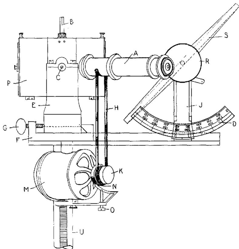
Elevation of Lummer-Brodhun with flicker attachment, motor, and neutral tint-absorbing screen, showing the method of clamping it to the head.
