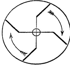
FIG. 6.—CROOKES RADIOMETER WITH SLANTING VANES.
